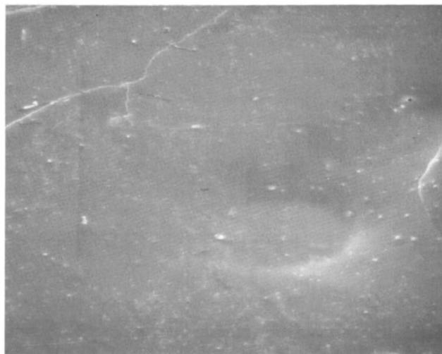
Figure 16. InP layer electrodeposited on a CdS substrate
